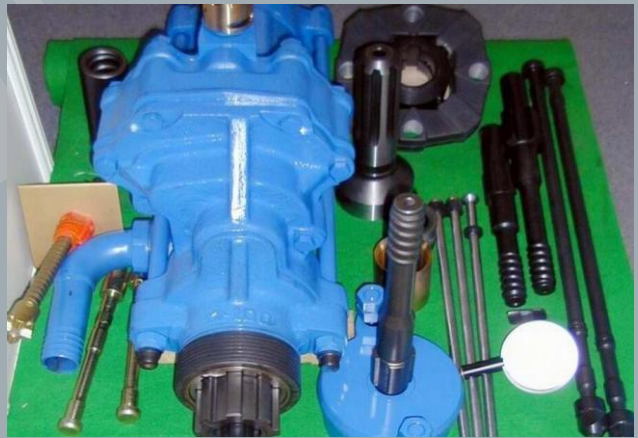
HYDRAULIC DRIFTER PREPARED FOR INSPECTION
