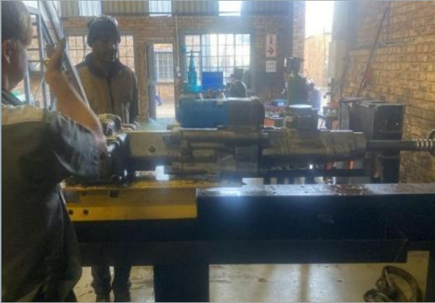
HYDRAULIC DRIFTER ON THE TEST BENCH BEING TESTED
